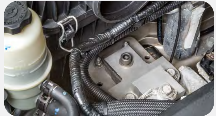
Load Cell Installed In Vehicle Engine Mount
